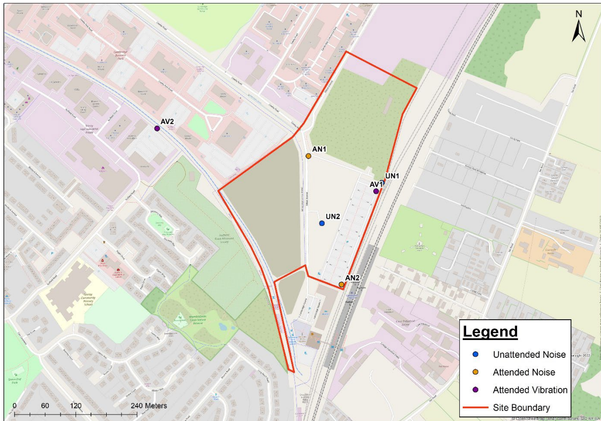
Figure A14.1.1 Survey measurement locations
