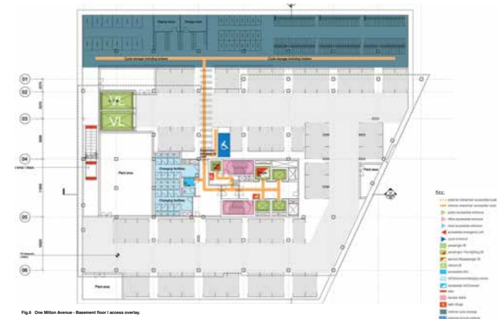
Fig 6 One Milton Avenue - Basement floor | access overlay.
