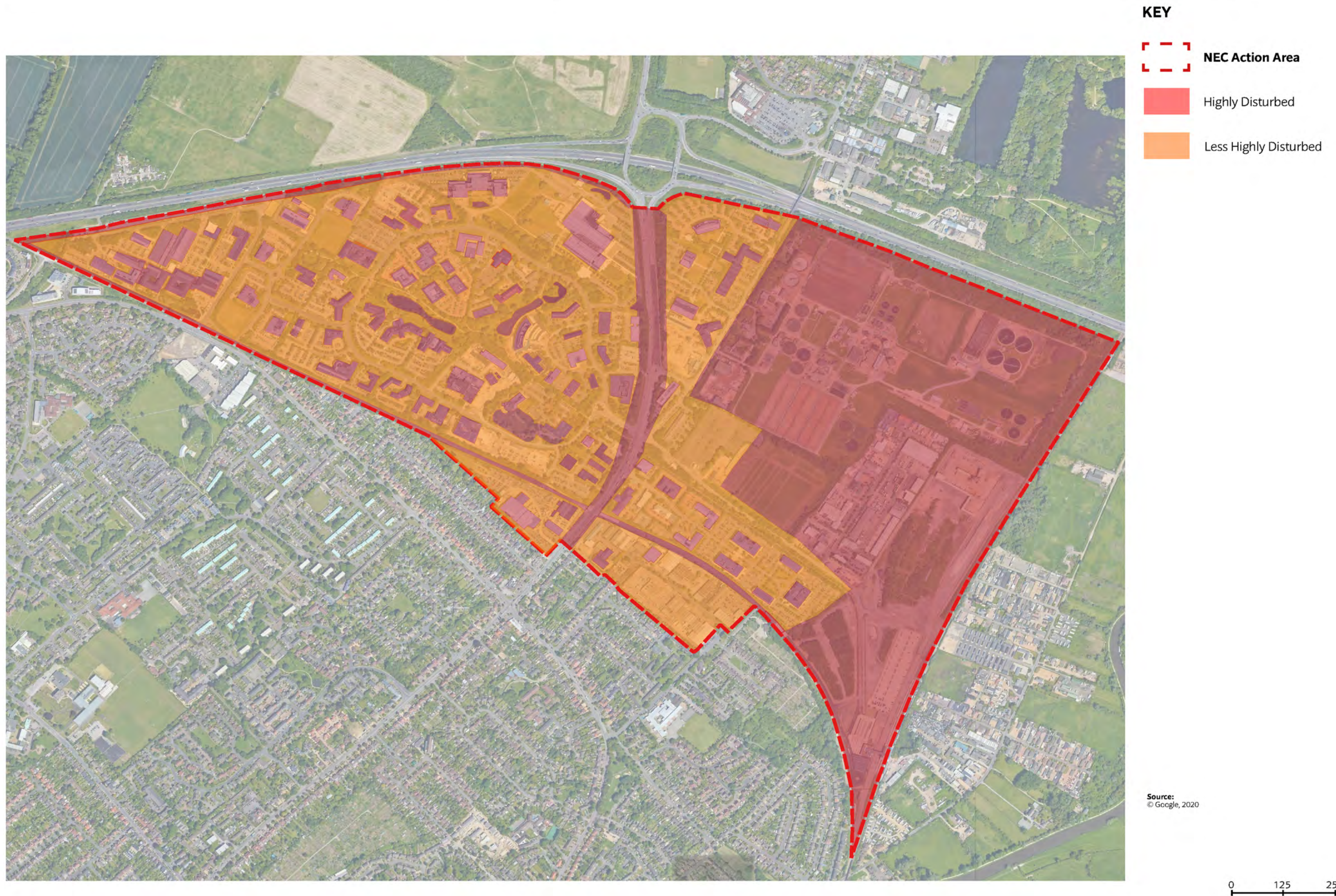
Figure 7: Likely ground disturbance
