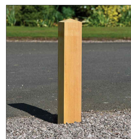
BO1 Proposed Timber Bollard | Supplier: Broxap | Product Code: BX17 Painted - Square | Dimensions: 150x150mm x1000mm | Fixing: Fixed into concrete footing. Reflective bands in rebates. Granite setts surrounded.
